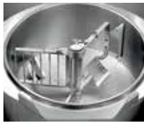
Mixing device with three arms - Removable
