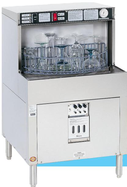
Model PKBR24 Batch Rotary Style glasswasher is easy-to-use and maintain. It has a convenient top-mounted instrument panel. The glassware is washed, sanitized and rinsed in removeable racks that move glasses in batches – saving handling time and broken glassware. Upper and lower spray arms incorporate fan-shaped spray nozzles that clean the entire glass both inside and out.
